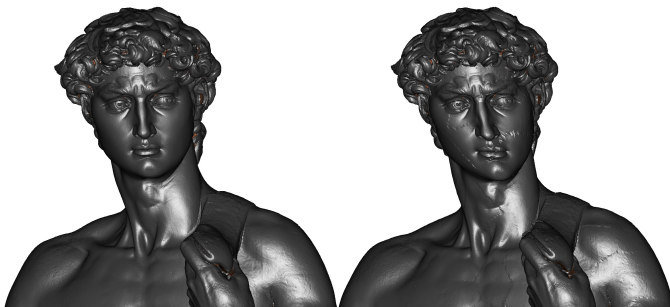
Figure 4: Correct mapping (left) and patching artifacts (right) generated by a wrong mapping configuration.
