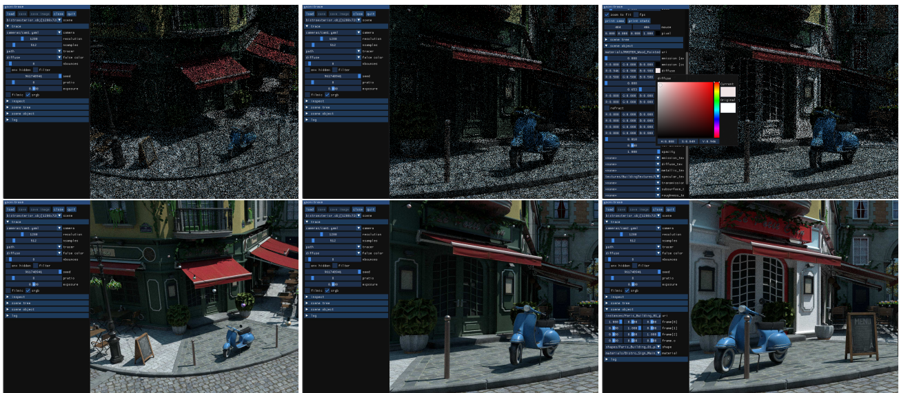
Figure 9: Example of interactive rendering and editing of large scene. (Left:) Our progressive path tracer gives immediately a low-sampled preview to allow real-time interaction. The image progressively converges as more samples are computed. (Middle:) The user can move the camera to interactively explore the environment. (Right) The scene can be edited in real-time, by changing materials and moving shapes. Model courtesy of Amazon Lumberyard [Lum17, McG17].
