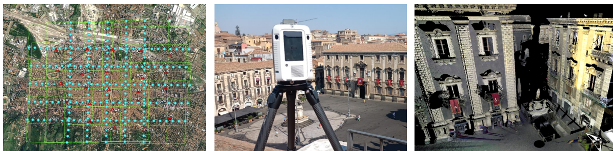
Figure 8: Left: extended area showing the aerial planning for aerophotogrammetric acquisition; middle: digitisation of the buildings of interest with fixed laser stations; right: partial scan. Image courtesy of START4.0.
