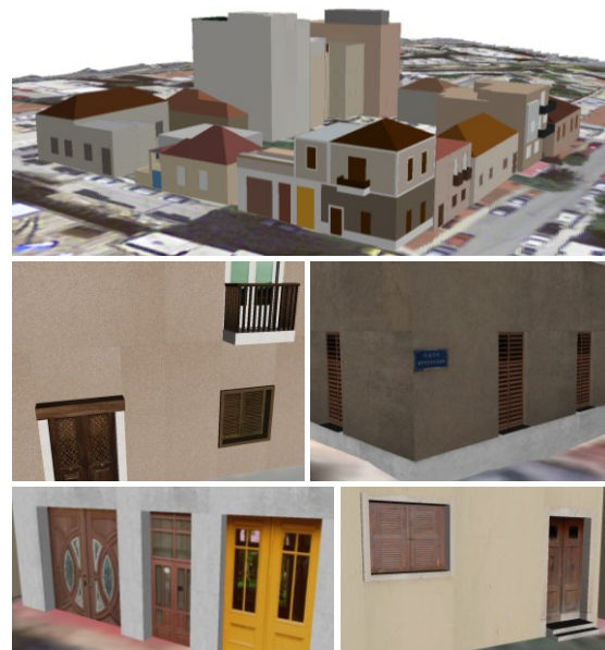
Figure 9: Top: 3D buildings of an urban block of Kessariani of 1983 at LoD2, superimposed on the DTM. Middle and Bottom: Details of the 3D models of 1983 at LoD3.
