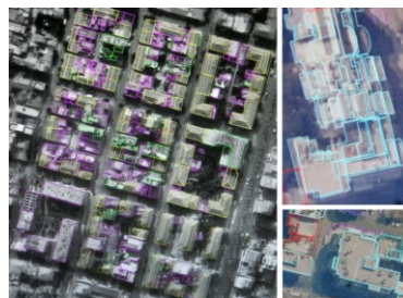
Figure 3: Stereo plotting of the study area using the 1983 and the 2010 stereo pair.
