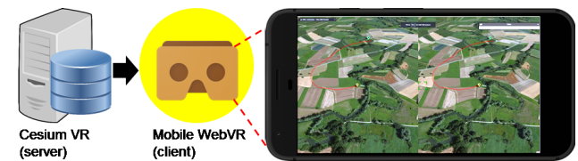
Figure 4: Stereoscopic visualisation of the bird trajectories using Cesium VR as implemented on the Chrome mobile browser.
