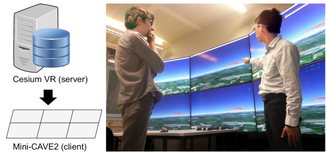
Figure 3: Stereoscopic visualisation of the bird trajectories using Cesium VR as a server and a tiled 3D display wall with polarised glasses as a display client.
