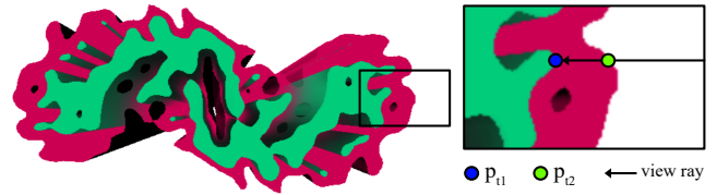
Figure 4: Depiction of two sample points p_{t_1} and p_{t_2} , which determine the intersection of the view ray and the fibril's surface and coat, defined by minimum density thresholds t_1 and t_2 , with t_1 > t_2 . Those thresholds are used to define the semi transparent coat to communicate model uncertainty of the underlying 3D reconstruction. As underlying density map, one 2D density map of the publication [SRL*15] is used.
