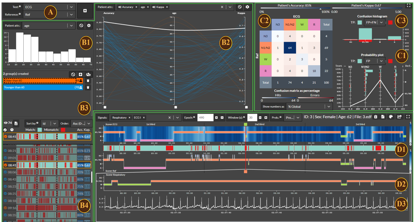
Figure 3: The views B1-B4 are patient-related, where B1 and B2 depict views where patients can be filtered based on the selections performed. B4 displays the patients that match the current selection. Groups of patients can be created, modified and selected in B3. C1-C3 shows performance information, where C1 depicts our probability plot, C2 a confusion matrix and C3 complements information displayed in the confusion matrix. In D1 the physiological data view shows the hypnograms for a selected patient. Alternatively, extra models can be visualized together with those the selected in A as shown in D2. Finally, D3 shows the signals that represent the input data.
