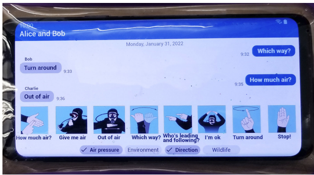
Figure 2: An image illustrating a novel communication method in terms of visual interaction for civilian divers underwater that utilizes a small number of diver hand-signal images as easily selected statuses and messages to be communicated. Source: [CCG22].
