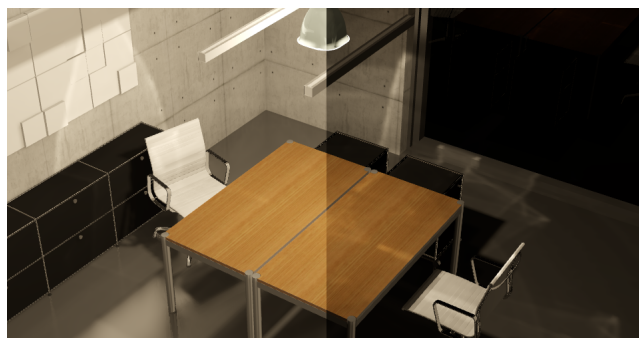
Figure 10: Comparison of the lighting produced by two different luminaires with different material properties and emission profiles, created with our luminaire editor, and imported into the light-planning software HILITE [VRV].
