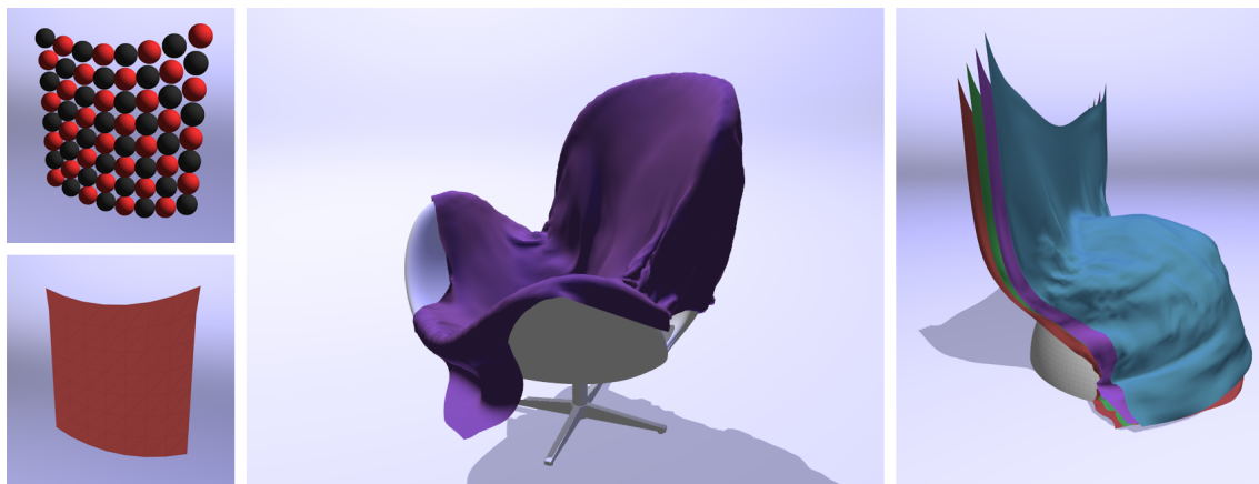
Figure 1: Left: a mass-spring network is partitioned into two independent sets of particles colored in red and black (top), and rendered as a triangulated mesh (bottom). During the animation, each one of these sets is efficiently computed in a single parallel step. Middle: a cloth-chair collision (19K springs, 2.5 ms per time step). Right: collision between four layers of clothes and a moving sphere (32K springs, 4.1 ms per time step). Timings include both numerical integration and collision handling.
