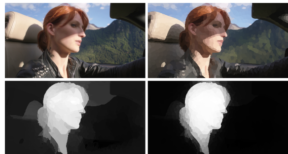
Figure 1: Saliency results on video. Top left: input video frame. Top right: superpixel segmentation. Bottom left: our per-frame saliency. Bottom right: final, temporally coherent saliency. Note how spurious, salient background elements on the car and sky are removed.
