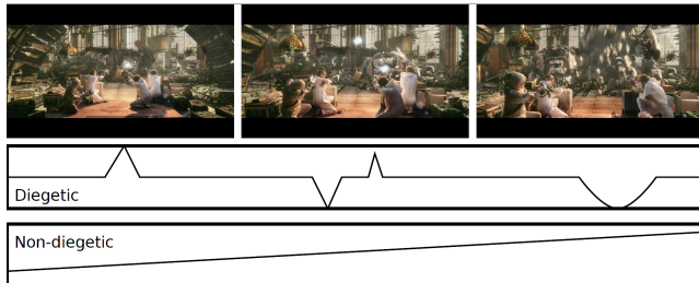
Figure 12: Example on Tears of Steel (07:53). A camera zoom is used to focus on the action and the coming characters. Soldiers try to shoot those characters. A diegetic haptic effect can be associated to the shoots to simulate the impact (top), or a non-diegetic haptic effect may be associated to the camera zooming to increase the dramatic intensity (bottom). ©Blender Foundation.
