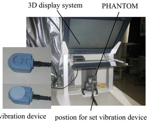
**Figure 2:** The system composed by 3D display and haptic devices.
