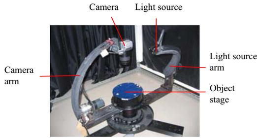
Figure 4: Optical gyro measuring machine (OGM).
