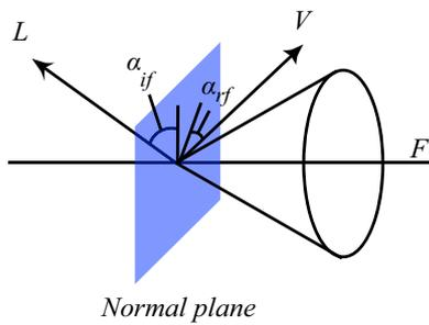
Figure 7: Rendering model of fiber in Japanese paper.
