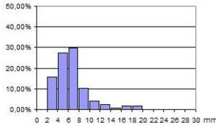
Figure 9: Mean Error (mm) Distr. for DB45R.
