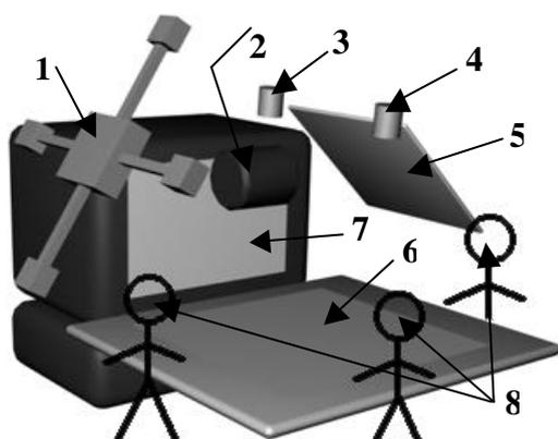
**Figure 1:** Visual Interaction Platform. 1-IS600 tracking device, 2-LCD Projector, 3-Camera, 4-Infrared light source, 5-Mirror, 6-Wacom Tablet (action-perception space), 7-Back projector (Communication Space), 8-Users
