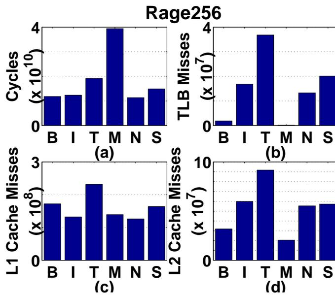
**Fig. 7.** Experimental results from the Rage256 data set. B = BONO, I = ISSUE, T = Interval Tree, M = Marching Cubes, N = NOISE, S = Seed Set/Surface Propagation.
