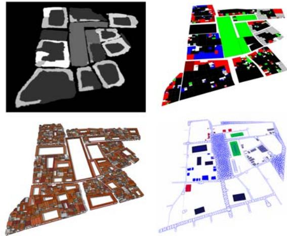
**Figure 6:** Four stages in the offline preprocess. Upper left: the manually designed map with five different gray levels for the building types. Upper right: output of the semantic part of the grammar (labeled footprints). Lower left: the output of the geometric part of the grammar. Lower right: the generated navigation graph from the combined grammar output.
