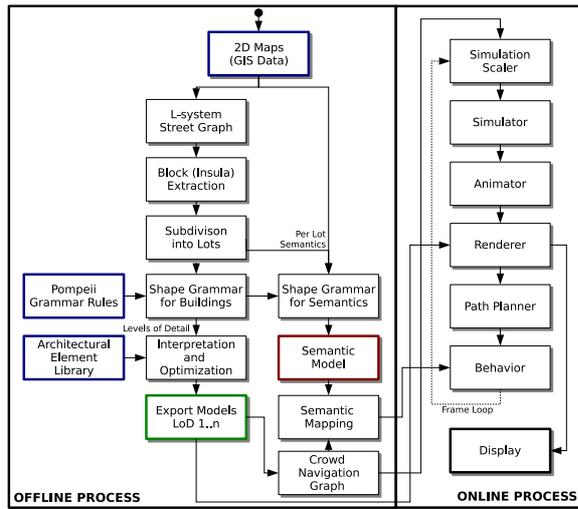
**Figure 3:** The overall pipeline consists of an offline and online part. The generation of the city model and semantics is done in an offline preprocess, where also the navigation graph is created and the behavior mapping is achieved. The online part deals with the scene rendering and the execution of the behavior actions based on character location.
