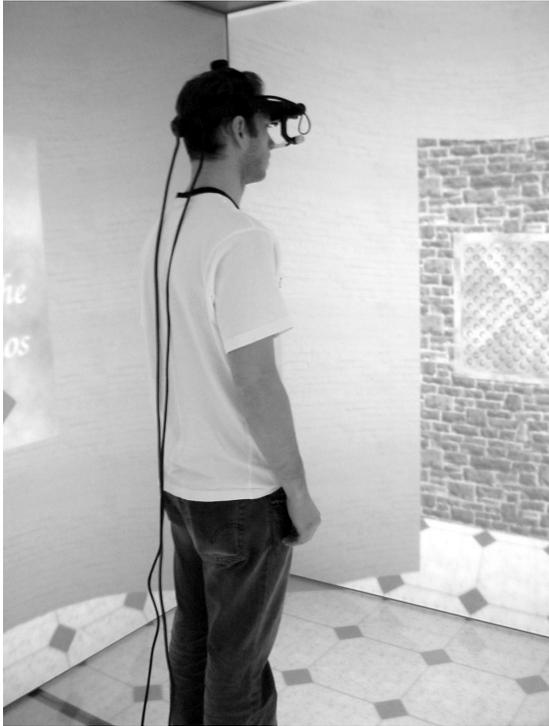
**Figure 1:** Eye-tracking system used in IVY, a six sided projective display located at York University [RLZ\*02].
