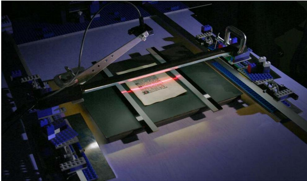
Figure 3.2: A linear light source (LLS) used to measure reflectometry. (picture: [37])
