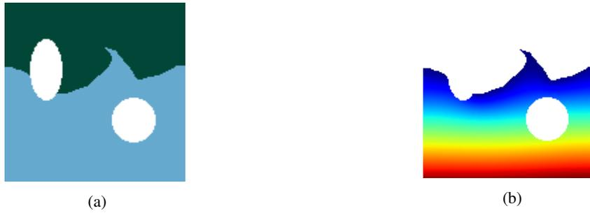
Figure 3.27.: (a) Two-dimensional domain for free-surface tests. Dark green areas correspond to Dirichlet boundaries, white areas to Neumann boundaries and blue areas to fluid. (b) Resulting pressure under gravity with colors indicating low pressure in blue to high in red.
