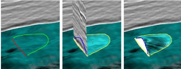
**Figure 6:** Creating a deformed fault in the horizon surface. The user sketches the cut, red line, and the region of interest, green line (left). The seismic volume is projected in the fault surface and the user draws the displacement, blue sketch (middle). Operator results (right).
