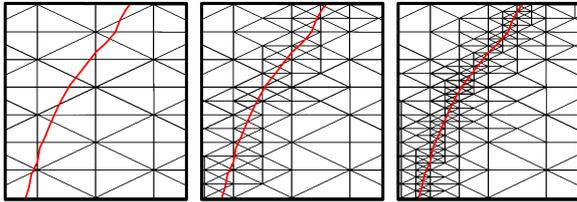
**Figure 9:** Sketch refinement. Sketch over the original mesh on left, and two approximations for different error values.
