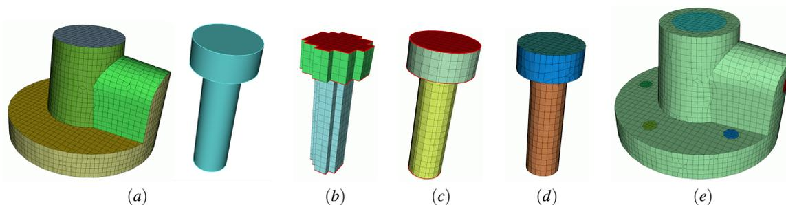
**Figure 1:** Insertion of a geometric element into an existing hexahedral mesh. In (a), the reference mesh  $M$  and the geometric element  $G_2$  to be inserted; in (b), cells of  $M$  that will be in  $G_2$  are selected and curves and surfaces classification is done; in (c), nodes are projected onto  $G_2$  while a sheet is inserted to improve mesh quality in (d). In (e), several imprintings have been performed to enrich the reference mesh.
