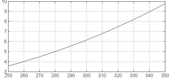
Figure 3: Heat flux in  $\text{Wm}^{-2}$  between two infinite walls whose temperatures differ from 1 degree
