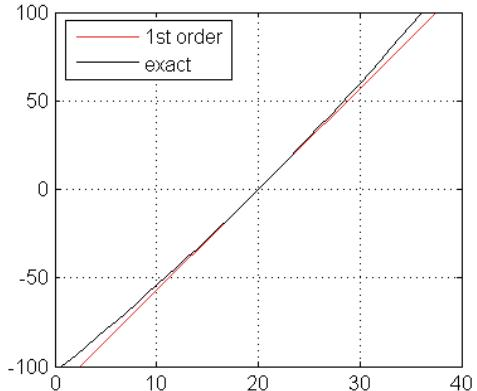
Figure 2: Transmitted power in  $W m^{-2}$  according to Stefan-Boltzmann law and its 1<sup>st</sup> order approximation computed in the region of 20°C, (293.15 K)
