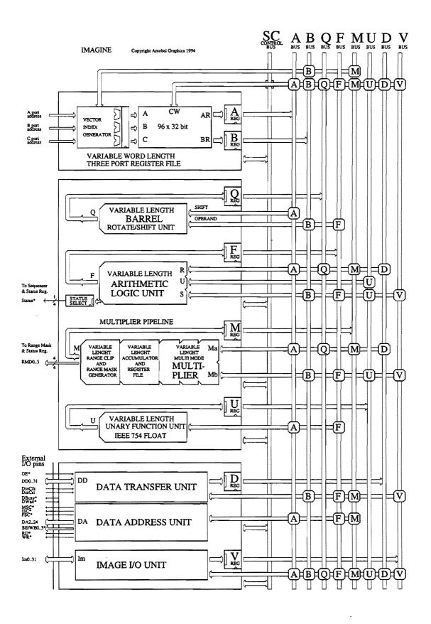
Figure 2: Data Processing Units of the IMAGINE .
