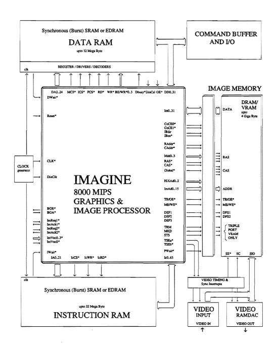
Figure 1: System Concept: IMAGINE plus external memories.
