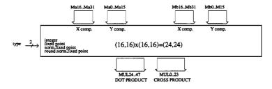
Figure 3: Multiplier modes (32 bit, double 16 bit and quadruple 16 bit).
