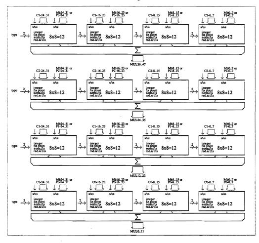
Figure 4: Multiplier modes (quadruple 8 bit and 16 fold 8 bit).
