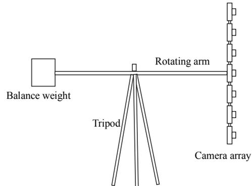
**Figure 2:** The setup of the capture system.
