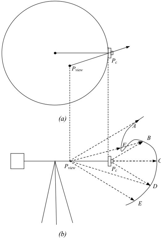
**Figure 1:** The problems in concentric mosaics method. (a) Top view. (b) Side view.
