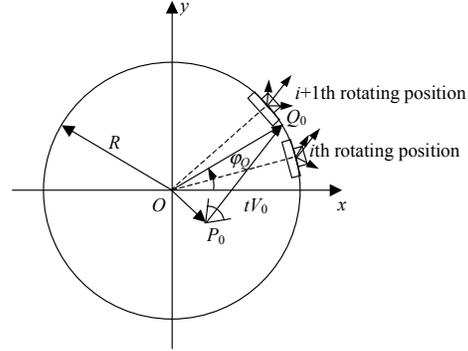
**Figure 6:** The determination of the rotation angle of the camera array.
