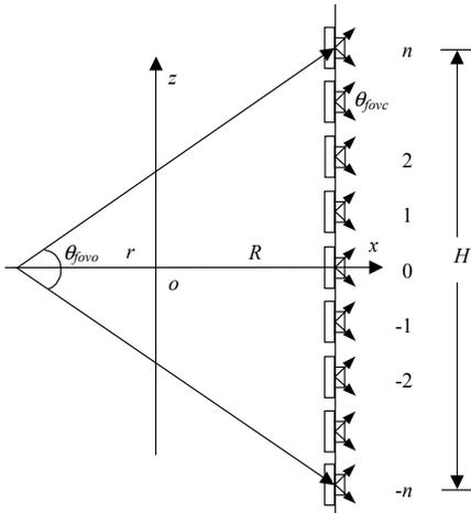
**Figure 4:** The relationship between the height of the camera array and the longitudinal field of view of the observer.
