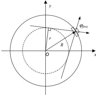
**Figure 3:** The relationship between the radius of the wandering circle and the lateral field of view of the capture camera.
