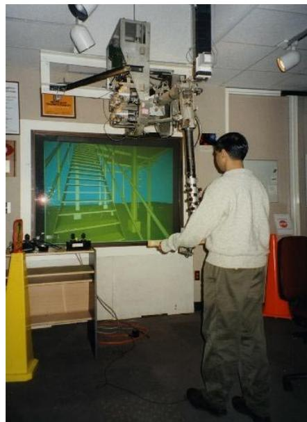
Figure 2: Projection screen and Argonne Arm
