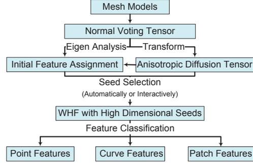
**Figure 2:** The functional pipeline of our new method. We use normal voting tensor to distinguish weak features from noise, and design anisotropic diffusion to determine different types of features.
