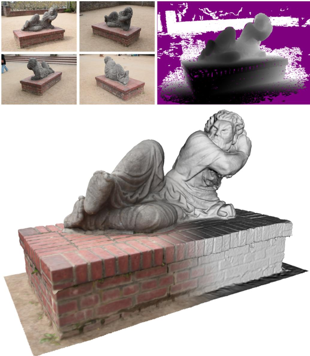
Figure 3.11: The *Der Hass* dataset. The top row shows 4 out of 79 input images and a depth map. The bottom row shows the reconstruction with and without color.
