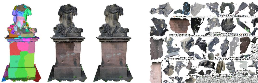
Figure 2.27: *Left:* The input geometry with the individual regions each colored by one view, the textured result before applying seam leveling, and the final textured result. *Right:* The final texture atlas produced by [Waechter et al. \[2014\]](#).
