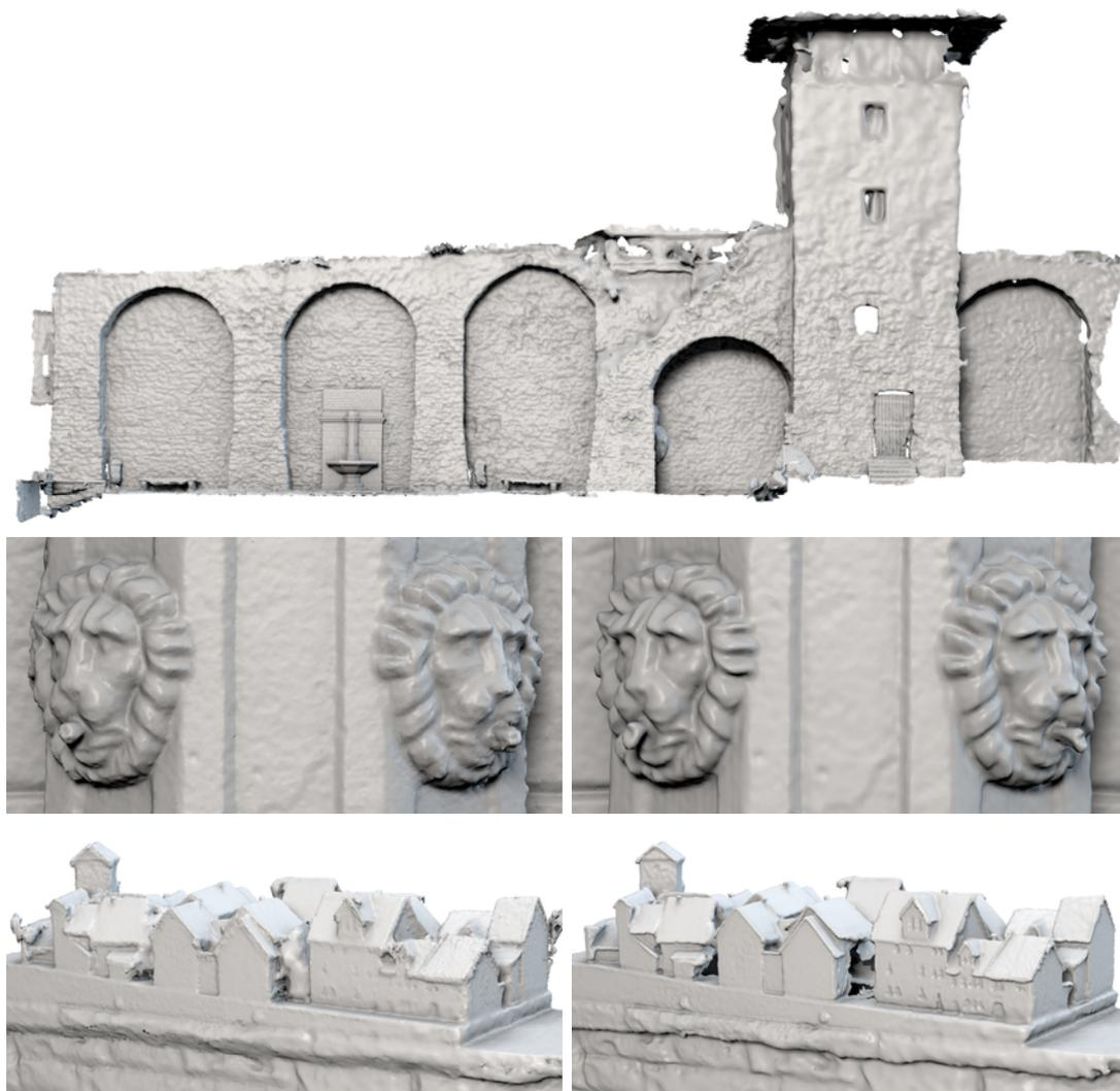
Figure 7.9: *Top row*: The full *Citywall* dataset without color reconstructed with *FSSR*. The fountain region is covered with more close-up input photos and a higher resolution mesh is extracted in this region. *Bottom rows*: Comparison of details reconstructed with *DMFusion* (left) and *FSSR* (right).
