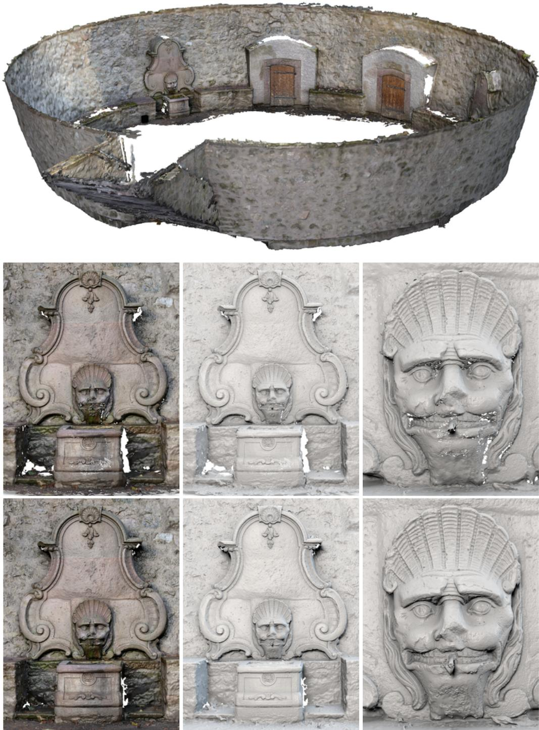
Figure 7.10: Comparison of the *Goethe Fountain* dataset. *Top*: The full reconstruction using *FSSR*. *Middle Row*: Details reconstructed with *DMFusion*, *Bottom row*: Details reconstructed with *FSSR*.
