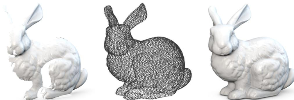
Figure 2.22: *Left*: A single triangulated range image only covers parts of the surface and multiple range images need to be fused to model an object. *Middle*: Surface samples are used as input for point-based reconstruction algorithms. *Right*: A reconstructed surface mesh.
