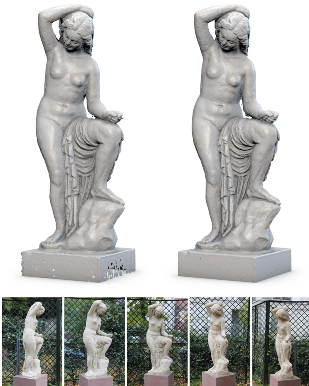
Figure 7.7: Reconstruction comparison of *Die Badende*, an uncontrolled MVS dataset with moderate scale differences. The bottom row shows 5 of the 343 input photos. The *FSSR* reconstruction (right) shows more detail and more complete geometry compared to the *DMFusion* reconstruction (left).
