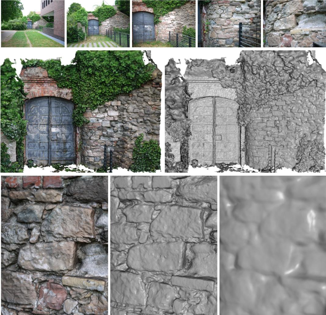
Figure 4.11: The top row shows some input images from the *Stones* dataset, and the middle row shows the reconstructed scene. The bottom row shows a close-up view of our reconstruction with and without texture (left, middle), and the corresponding VRIP reconstruction (right).
