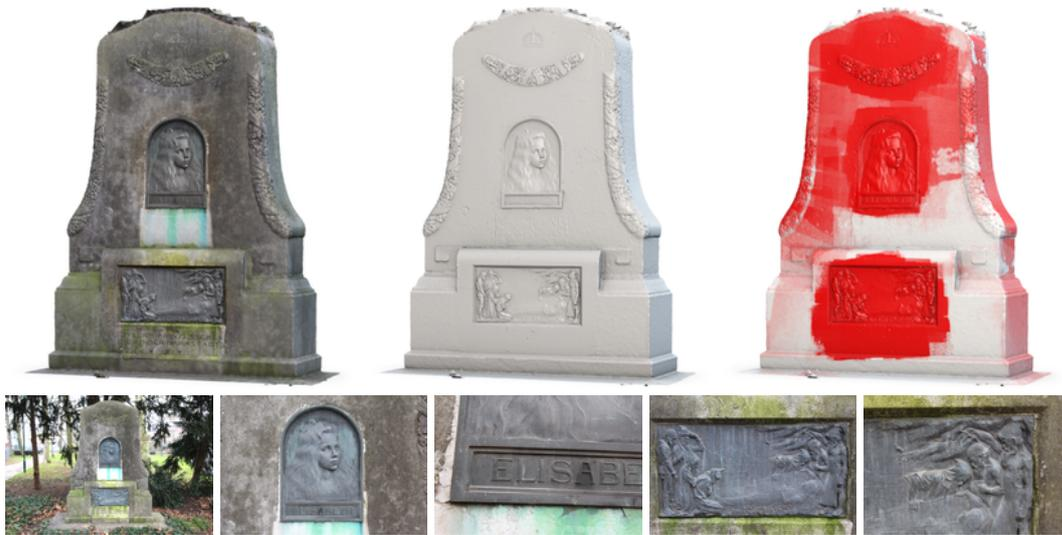
Figure 5.14: Multi-scale reconstruction of the *Elisabeth* dataset. The top row shows our reconstruction with color (left), with shading (middle) and with false coloring of the scale (right). The bottom row shows 5 of 205 input images with varying scale.
