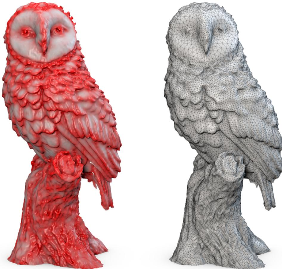
Figure 7.13: The *Snow Owl* reconstruction with 280 727 vertices (left, density field shown) is remeshed to 25 000 vertices with an adaptive vertex distribution. Regions with low curvature receive fewer triangles, such as the face region. Given a predetermined vertex budget, this leaves more triangles for regions of higher curvature to increase fidelity to the original surface.
