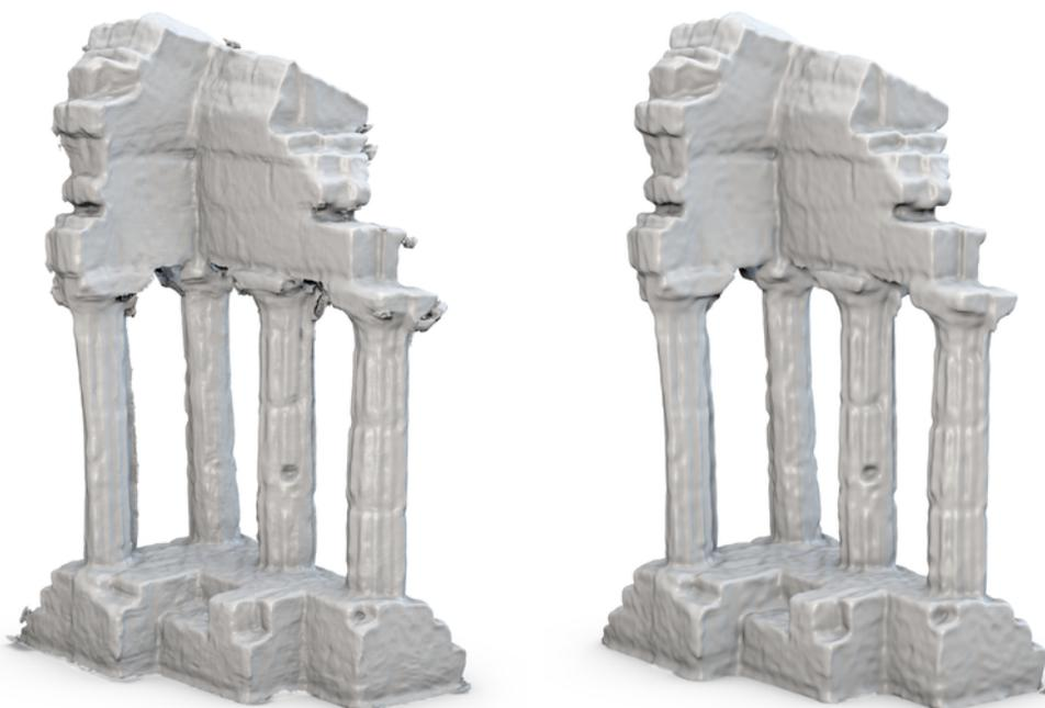
Figure 7.5: Reconstruction of the *Middlebury Temple* with *DMFusion* (left) and *FSSR* (right). Although the *DMFusion* reconstruction produces slightly sharper edges in some regions, the *FSSR* reconstruction is very clean without spurious geometry.
