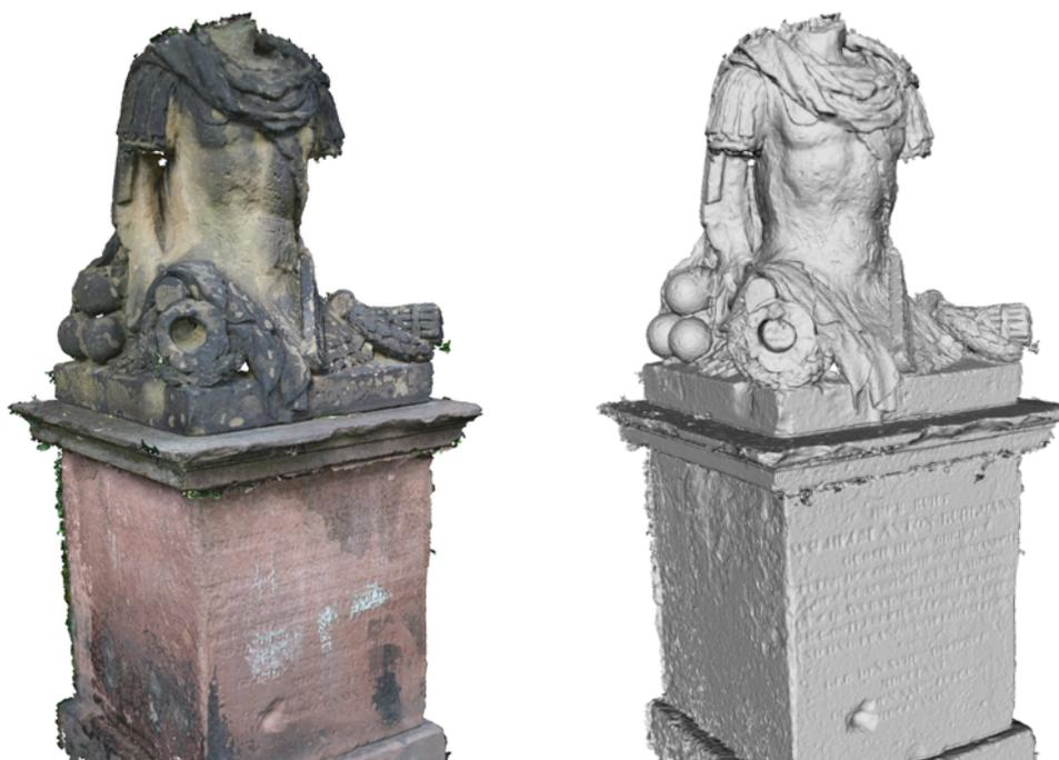
Figure 3.5: The final surface reconstruction with color (left) and shaded (right). Notice how even the engraved text is visible in the geometry.
