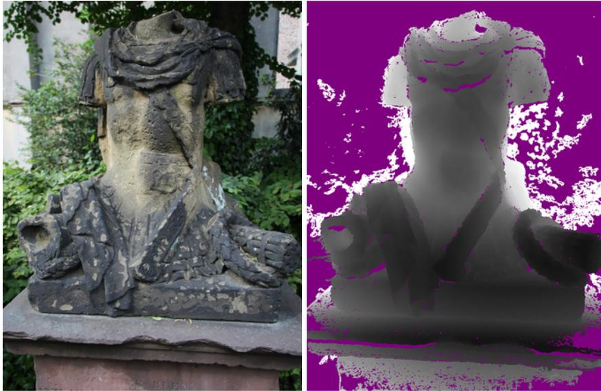
Figure 3.4: An input image and the corresponding depth map reconstructed with multi-view stereo. Each depth value encodes the distance from the camera.
