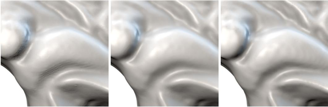
Figure 7.2: *Left*: The reconstruction of the *Polymetric Dragon* with *DMFusion* shows a few small artifacts. *Middle*: Performing the *DMFusion* reconstruction on a single scale removes these artifacts. *Right*: The reconstruction using *FSSR*. Note: All images are contrast enhanced.
