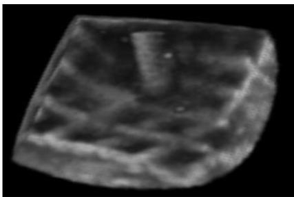
**Figure 3:** Above shows the 2D image of the entire grid and guide-wire for 3D-FV rendered on the SONOS 7500's CRT display. Keyboard and mouse were used to change viewing angles. For 2D-RT and 3D-RT, only a 2D slice or a section of the above full-volume sector could be seen, and manipulation of the ultrasound transducer was needed to change viewing angles.
