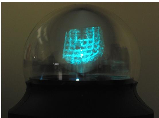
**Figure 4:** Perspecta's display of the entire phantom is shown. In most cases, a tilt of the user's head was all that was needed to get desired perspective. Anyone can view the same volume from all around display.
