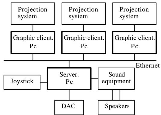
**Figure 1:** first prototipe.
