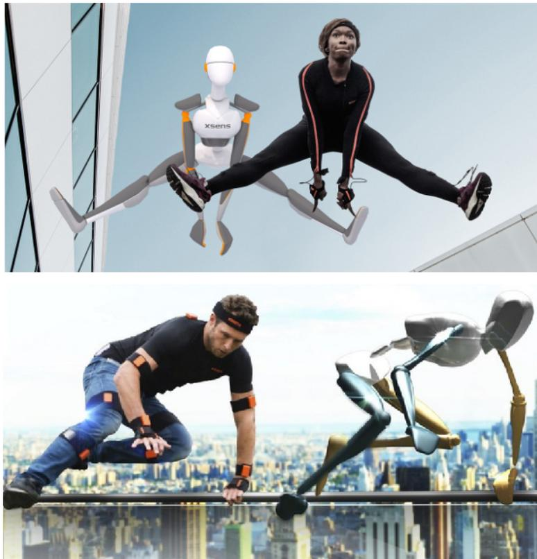
FIGURE 2.4: Inertial motion capture systems. Top: Sensors are integrated into a suit. Bottom: Individual sensors are attached to the performer.
