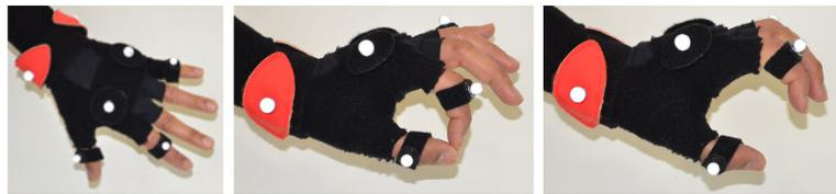
FIGURE 3.2: Marker setup for finger motion capture. (Image by Vicon®)
