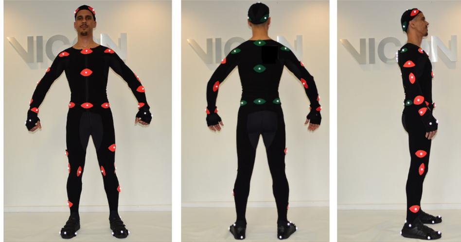
FIGURE 3.1: Marker setup for body motion capture. (Image by Vicon®)
