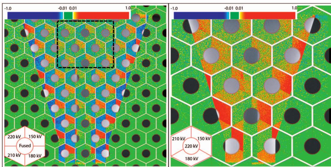
Figure 1.7: Example for a *superposition*. Slices of volume datasets can be compared by subdividing the image space into hexagonal regions. Each of these region is then subdivided into smaller elements that depict data from different volume slices [MHG10].
