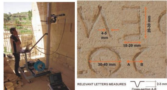
**Figure 2:** The triangulation-based range sensor mounted on a mobile motorized structure (left) and the relevant letters measures on the Great Inscription (right).
