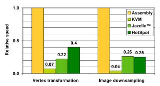
Benchmarked on an ARM926EJ-S processor with hand-optimized Java and assembly code
