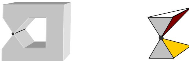
**Fig 14:** Non-manifold solid with a non-manifold edge (left) and vertex (right).
