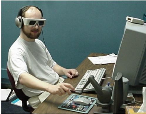
Figure 5: GDIS uses stereographics, haptic force feedback and sonification.
