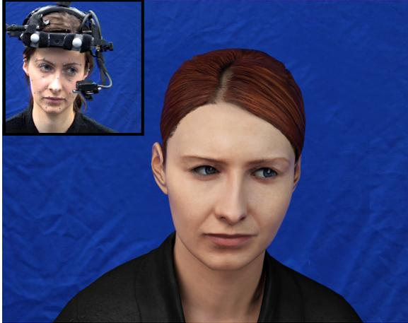
**Figure 5:** Eye movement capture using a head-mounted eye-tracking device, and corresponding virtual avatar displaying the recorded eye-movements [MBB12]
