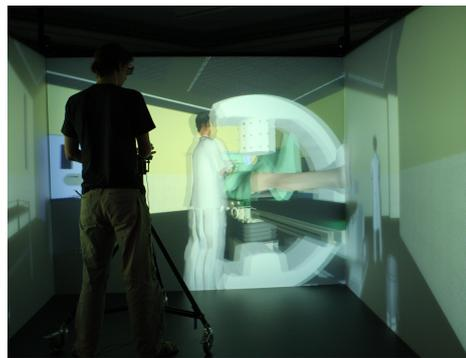
**Figure 1:** Running the surgery workflow simulation in a CAVE using stereoscopic projection.
