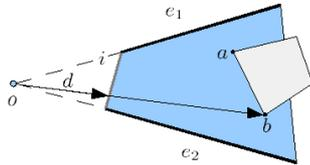
**Figure 2:** A beam is defined by four edges. The two edges  $e_1$  and  $e_2$  form a quadrilateral whose baseline  $i$  we call the image plane of the beam. The point  $o$  is the (virtual) origin of the beam. A ray  $r = o + \lambda d$  is constructed through the image plane and intersected with the face  $\{a, b\}$  which was identified in the beam framebuffer.
