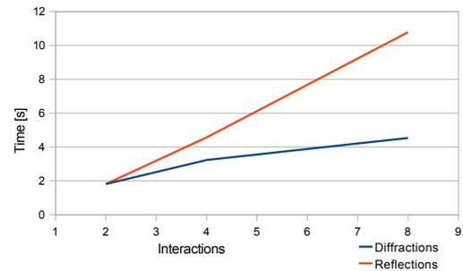
**Figure 6:** Performance of our algorithm for varying levels of interactions. Computation complexity grows approximately linearly in the number of reflections.
