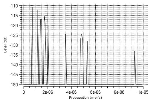
**Figure 9:** A simulated delay spread histogram for one receiver position in the Munich scenario. The multiple peaks represent different propagations paths, which arise due to reflection and diffraction.
