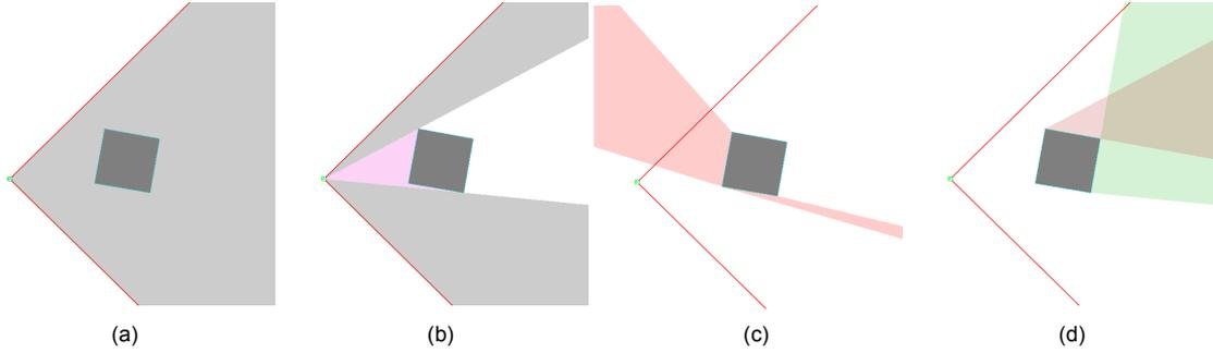
**Figure 3:** (a) A beam is created and intersected with the geometry. (b) The beam is split into child-beams, according to the intersections. (c) Reflection edges are identified, and the old beam origin is reflected at those edges, constructing reflected beams. (d) In the same manner diffraction beams are generated at silhouette edges.
