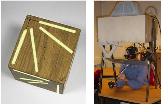
**Figure 1:** (left) An example 7x7x7cm input device with line pencil fiducials. (right) A prototype Personal Space Station.
