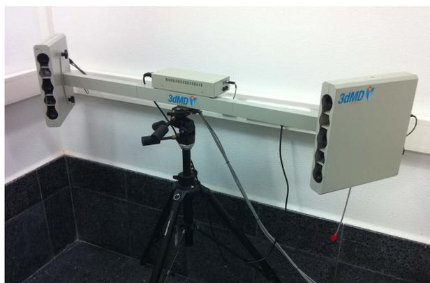
Figure 1.5: 3dMface System, used in face scanning.
