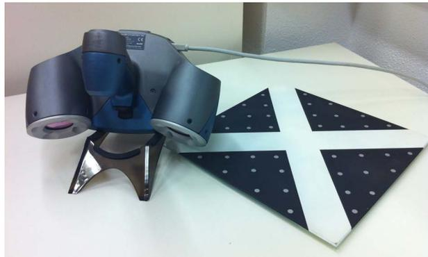
Figure 1.6: Creaform REVscan laser scanner, used in reverse engineering.
